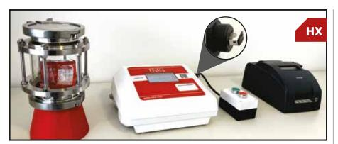
The H5K5.HX is a non-destructive leak tester, investing in it is easy to justify as it reduces material waste and guarantees product quality considering that the samples that pass the leak test can be put back on the production line.
